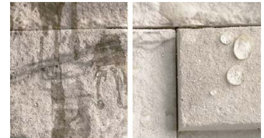
Hydrophobic surface with water repellent coating
