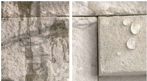
Hydrophobic surface with water repellent coating
